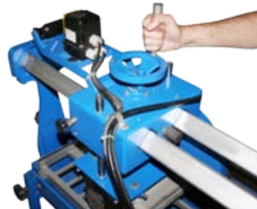
Manual depth adjustment of cutting head by hand wheel.
